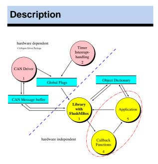
The *CANopen Library* consists of a hardware independent and a hardware dependent part that communicate with message queues. The hardware dependent part consists of controlling software for the CAN controller and timer functions. A detailed description can be found in the *CANopen Driver Package*.
