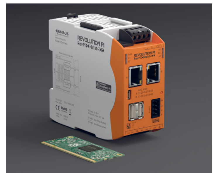
At 45mm, the RevPi Connect is twice as wide as the RevPi Core 3.
