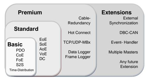
**Cable Redundancy** - in case of cable or device failure the function ensures the network segments go on with operation except those behind the failure.
