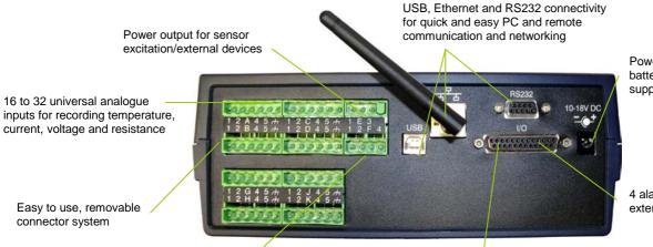
Power supply – internal alkaline batteries or external DC power supply
