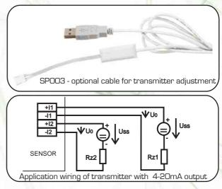
Included accessories - Traceable calibration certificate from the manufacturer, instruction manual. Calibration certificate with declared metrological traceability of etalons is based on requirements of EN ISO/IEC 17025 standard. Free program TSensor for configuring of the transmitter is ready to download from www.cometsystem.cz
