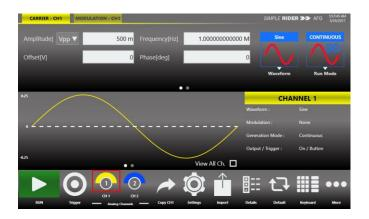
Simple Rider UI is designed for touch and it has been developed to put all the capabilities of modern Waveform Generators right at your fingertips. All instrument controls and parameters are accessed through an intuitive UI that recalls the simplicity of Tablets and modern smart phones: touch features and gestures are available to engineers and scientists to create advanced waveforms or digital patterns in few touches.
