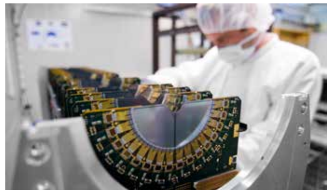
CERN - Assembling the last module of the vertex locator for LHCb. Photograph: Maximilien Brice. © 2007-2017 CERN. All Right Reserved.
