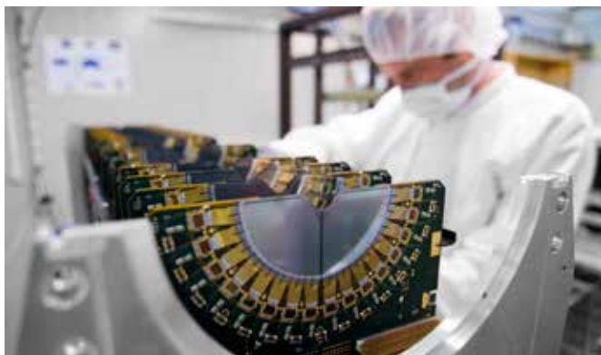
CERN - 为底夸克实验（LHCb）装配最新的顶点定位器模块。图片：Maximilien Brice. © 2007-2016 CERN. All Right Reserved.
