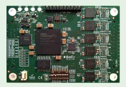
SoCe offers a carrier, SMARTcarrier, that can be used by the customers as a reference to design their own one or to include SMARToem in their equipments.
